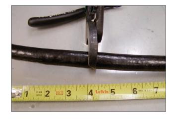
2. Cut into the top braid layer approximately one inch and remove the excess top braid layer.
