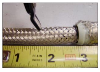
5. Slide a neutral banging split ring (PART B) underneath the internal braid layer.
