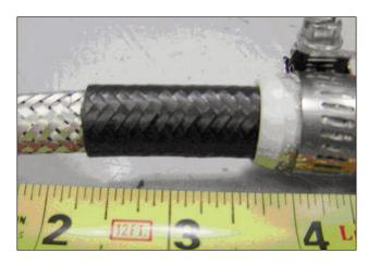
7. Leave approximately 1" of the internal layer of braid and remove the excess.
