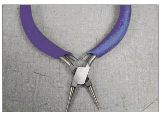
3. Take a ground banding split ring (PART A) and work it underneath the top braid layer. The braid layer should cover as much of the split ring as possible. It may be beneficial to use a tool as shown to open the braid layer making it easier to insert the split ring.
