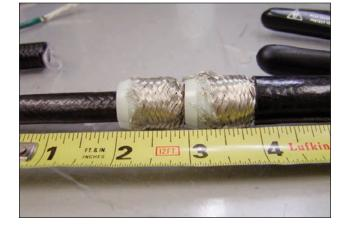
6. Strip a length of green ground conductor (PART F) sufficient to span the distance of both couplers (approximately 2 inches worth of stripped wire.
