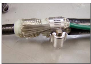
9. With both couplers securely tightened, the cable should resemble the picture shown.
