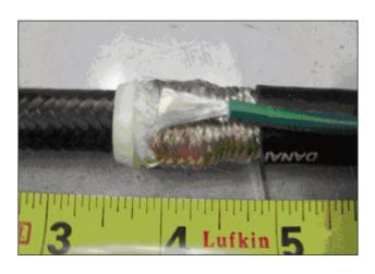
4. Strip the green ground conductor (PART F) approximately 1". Spread the leads out. Place it on the top braid layer as shown. Preform wire as shown.
