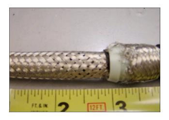
4. Cut back the second layer of insulation as close to the top insulator as possible. Move down one inch and cut around the internal braid layer. Remove the excess.
