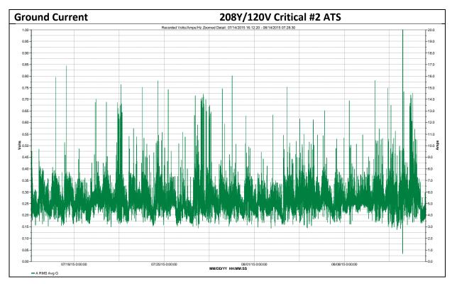
Large amounts of current flow on ground can adversely affect equipment and trigger ground fault circuitry. The ground current level indicates the likelihood of wiring errors in the distribution network supplied by the "Critical #2" ATS. Two common wiring errors are:
